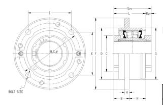
timken QVVCW19V085S Solid Block/Spherical Roller Bearing Housed Units-Double V-Lock Piloted Flange Cartridge
